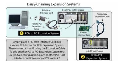
In the daisy-chain configuration, successive PCI expansion systems are added to the "end" of the PCI bus hierarchy, which adds "depth" to the PCI Local Bus by increasing the number of PCI Local Bus levels active in the system configuration.
